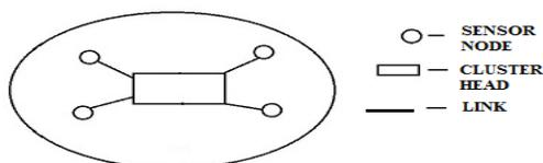
Figure 4: Structure of a Cluster
